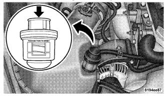
The clear plastic housing on the Filter Minder™ (If Equipped), allows you to view the amount of air pressure drop across the filter element. It consists of a diaphragm and a calibrated spring sealed inside the plastic housing. As the air cleaner filter becomes clogged and air pressure drop across the filter element increases, a yellow disc travels along a graduated scale on the side of the Filter Minder™.
